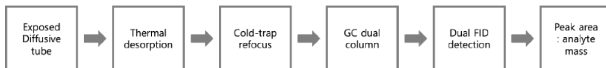
Figure 2.6.2 Analytical workflow from an exposed diffusive tube to quantified analyte mass under thermal-desorption GC-FID.
