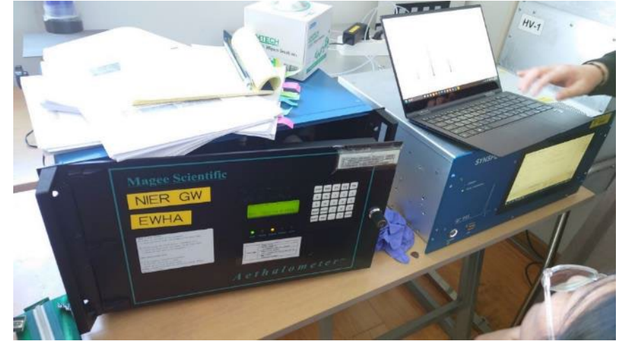
On-line BC monitor (left) and VOC monitor GC-PID (right) from Ewha Womans University, Korea
