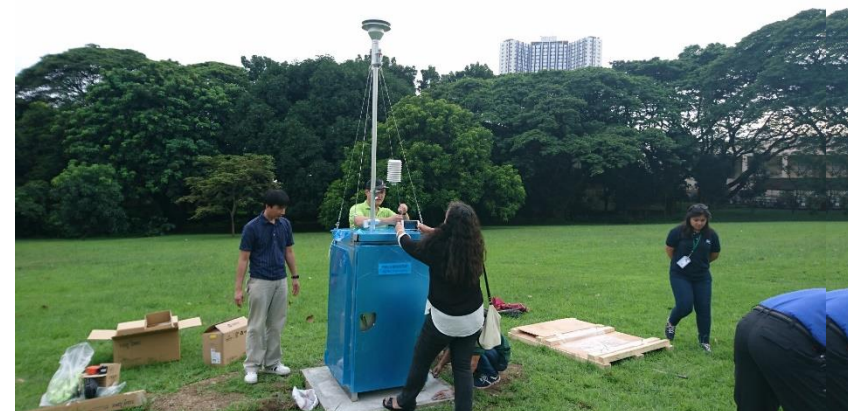
Installation of automatic PM2.5 monitoring equipment in the Philippines in 2017
