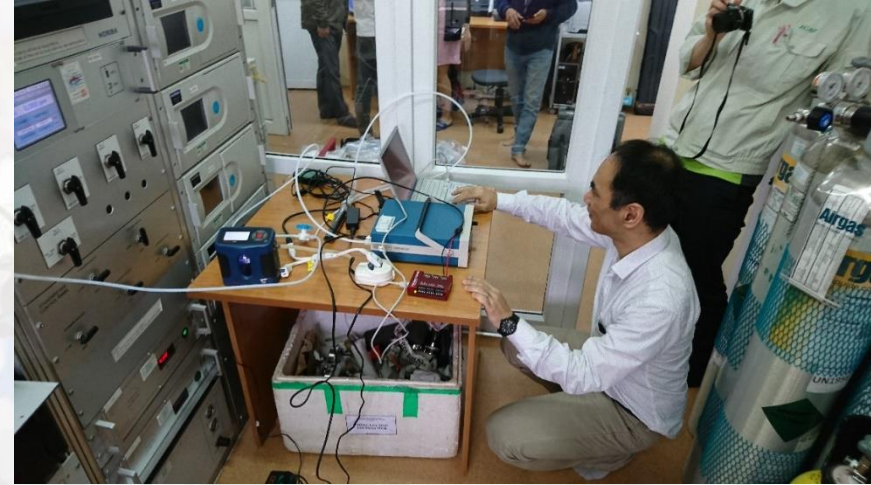
Ozone monitor calibration at Hanoi, Vietnam
