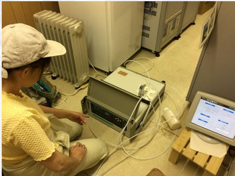
Ozone monitor calibration in Japan
