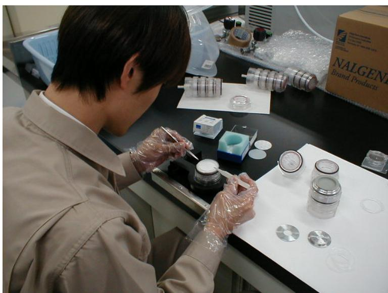
Mounting a filter on a stage
