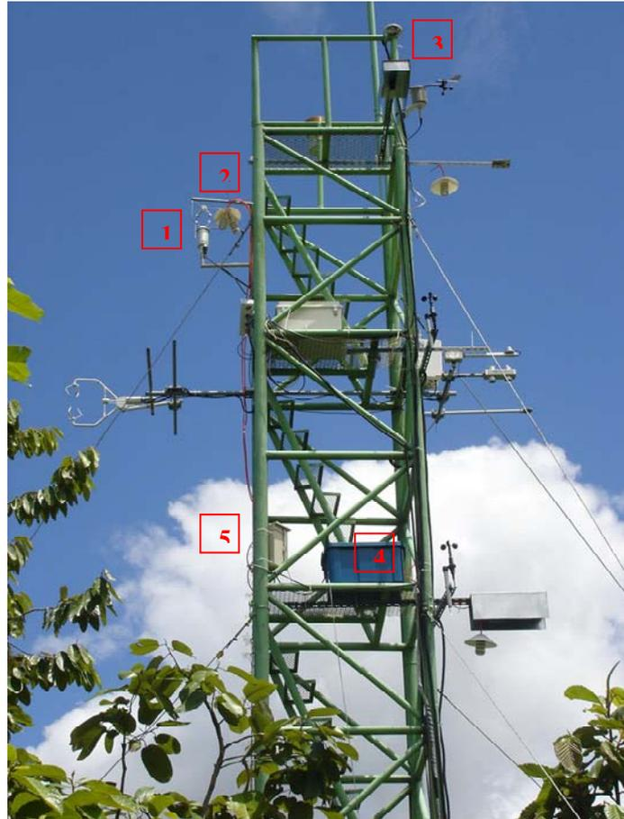
Figure 3. The experimental tower equipped with meteorological instruments consisting of 1. 3D ultrasonic anemometer, 2. filter packs, 3. Temperature and relative humidity sensor, 4. vacuum pump and 5. flow meter and solenoid valves.
