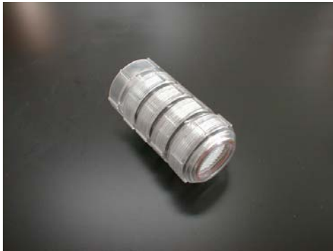
NILU filter holder (4 stage, open face)
